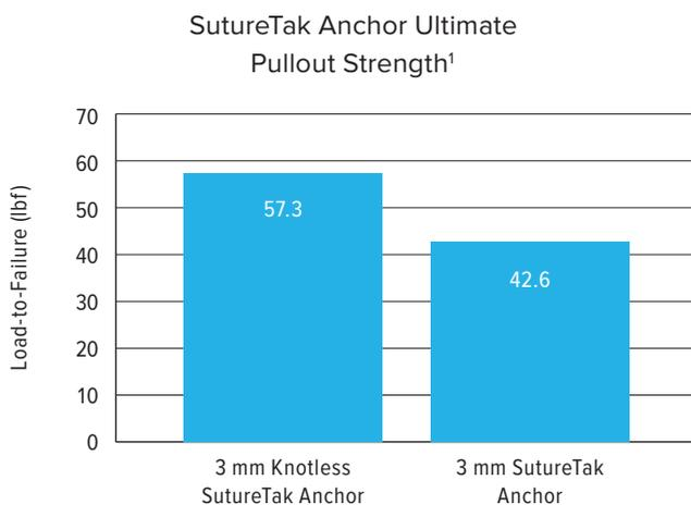
Failure mode: Suture pulled through anchor
