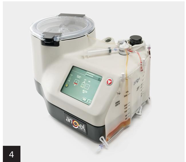
The Angel system first collects PPP. Collection will stop when the 470 nm wavelength of light is absorbed by platelets. The Angel system will adjust the valve position to collect PRP until red blood cells are detected by the absorption of the 940 nm wavelength of light.
