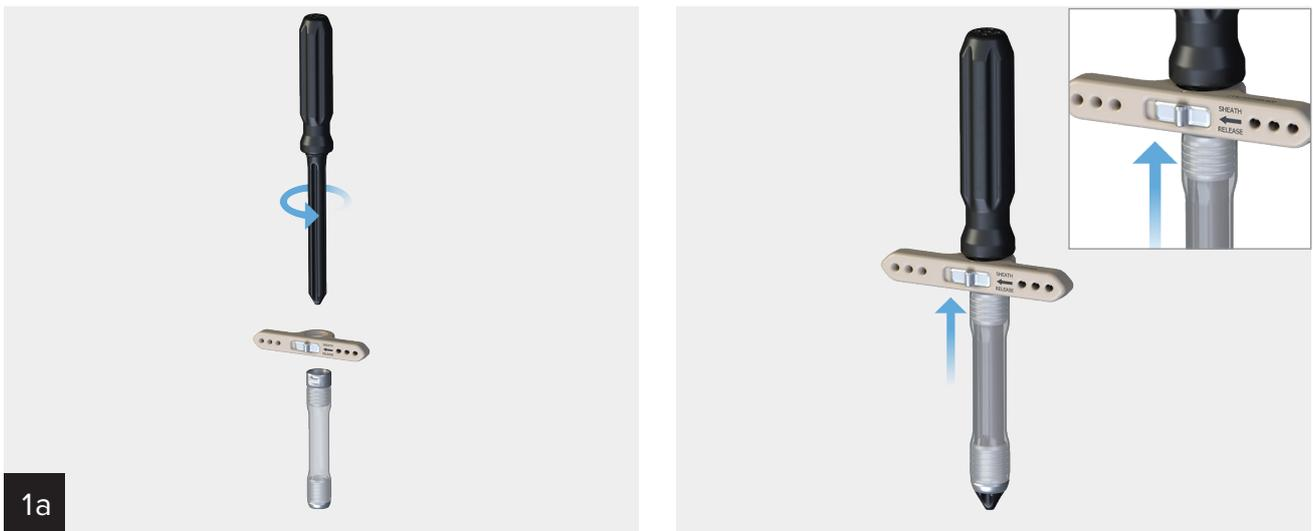
Assemble the pin guide, sheath handle assembly, and suprapatellar entry sheath.
