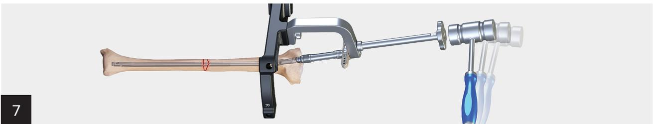
Insert the nail over the ball nose guidewire and into the canal. If the nail does not enter the tibia easily, use a slotted mallet to strike against the impactor pad surface.
