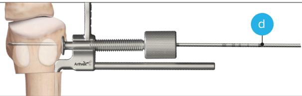
**Trajectory guide**—sets trajectory of the K-wires relative to the position of the capital fragment guidewire
