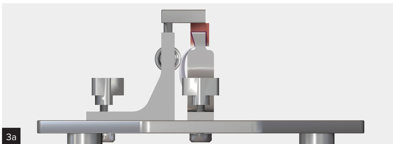
Secure cutting guide #1 into the workstation and position it so the vertical cutting face is aligned with the vertical face of the holding post. Use a sagittal saw to complete the cut.
