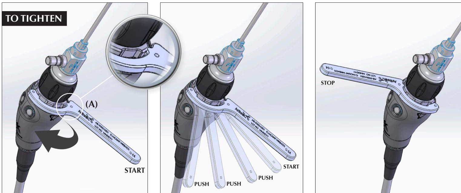
**To tighten the scope on the head:** Screw the scope on to the Synergy<sup>UHD4™</sup> C-mount camera head by hand until tight. Place the wrench on the silver nut (A) on the scope. While holding the camera head firmly, **PUSH the wrench clockwise** to tighten the scope on the camera head.
