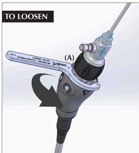
**To remove the scope from the head:** Place the wrench on the silver nut (A) and push the wrench counterclockwise until the scope is loosened. Continue unscrewing by hand to remove the scope.
