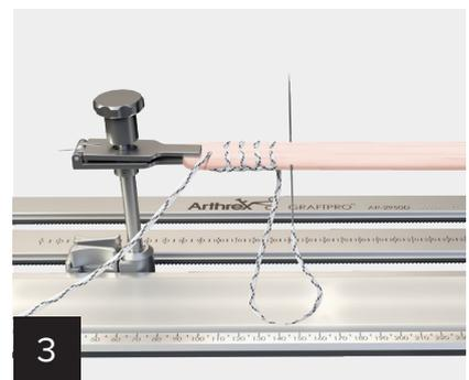
After creating several locking stitches down one side, the needle transverses the tendon. Create locking stitches down the opposite side of the tendon using the same technique. Leave the suture tails at the end of the tendon.
