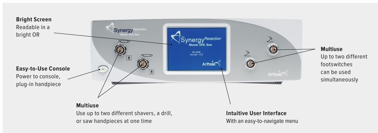
This versatile Synergy<sup>Resection</sup> system was designed for multiple orthopedic procedures and operates like two consoles in one chassis. It can simultaneously operate two accessory handpieces completely independent of each other. Operators can also use one or two foot pedals to control each of the accessory handpieces. Shaver handpieces offer three oscillating modes depending on the application or surgeon's preference: standard, efficient, or aggressive.
