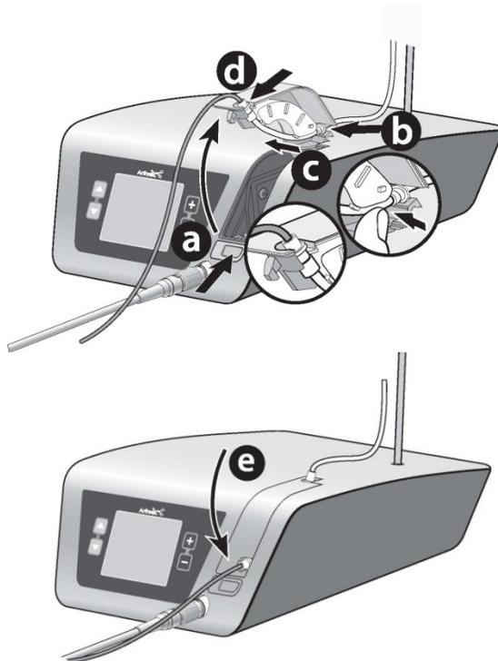
**Table 16 Irrigation Pump Tubing Configuration**
