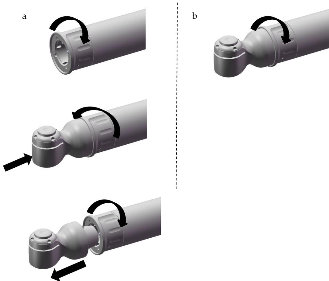
**Table 15** Connecting and removing an attachment
